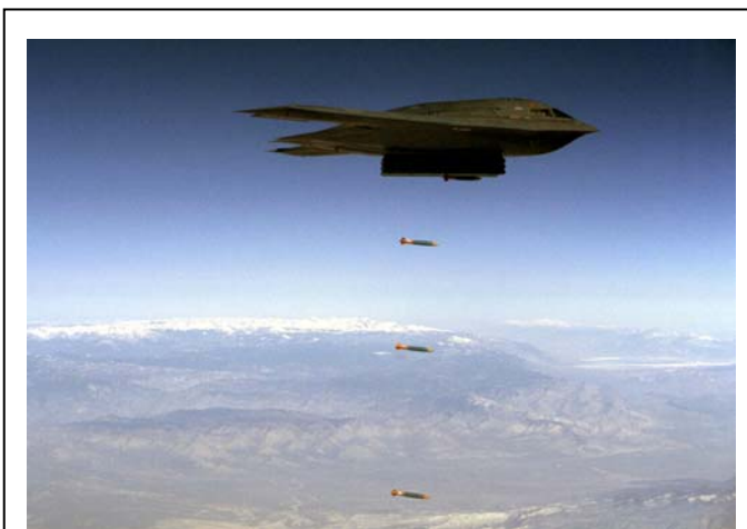
Figure 2: B-2 JDAM Release Test
